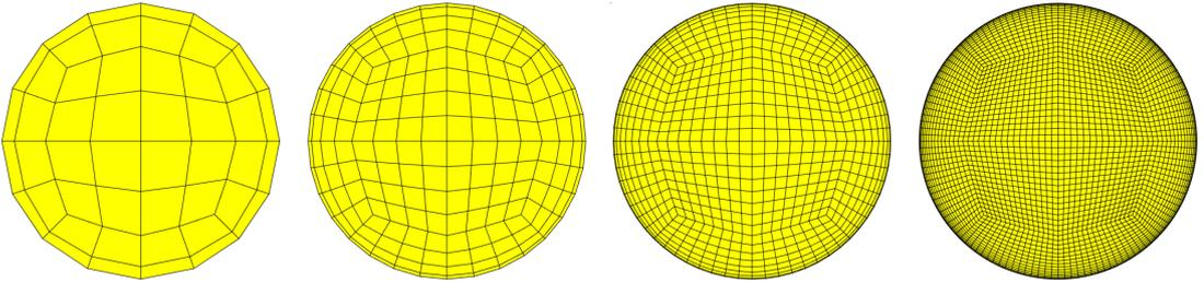
**Figure 11:** Frontal view of the graded meshes used for the Poiseuille flow problem.
