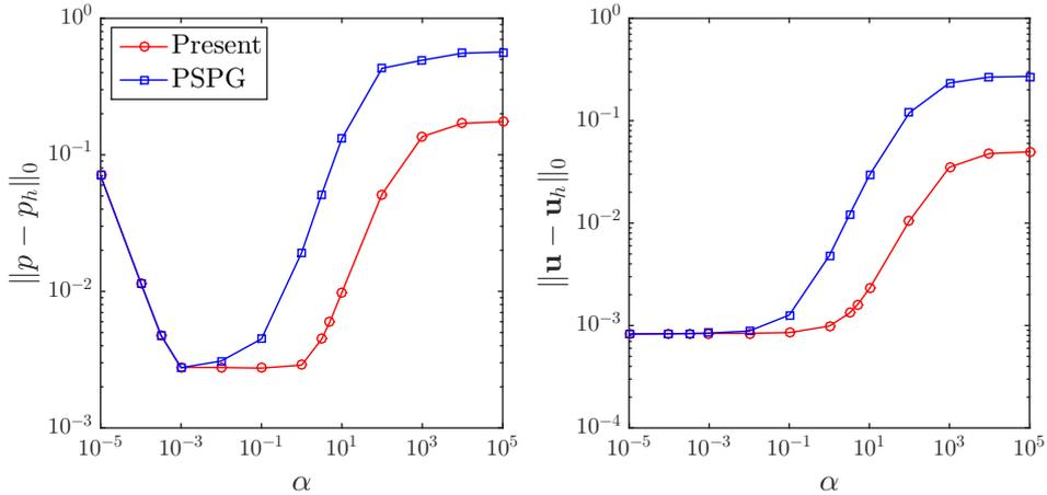
**Figure 7:** Kovaszny benchmark: error with respect to stabilisation parameter.
