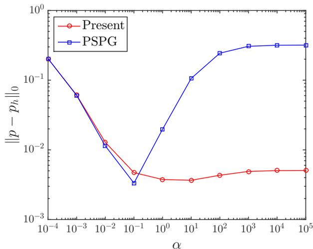
**Figure 2:** Stokes problem: pressure error with respect to stabilisation parameter.
