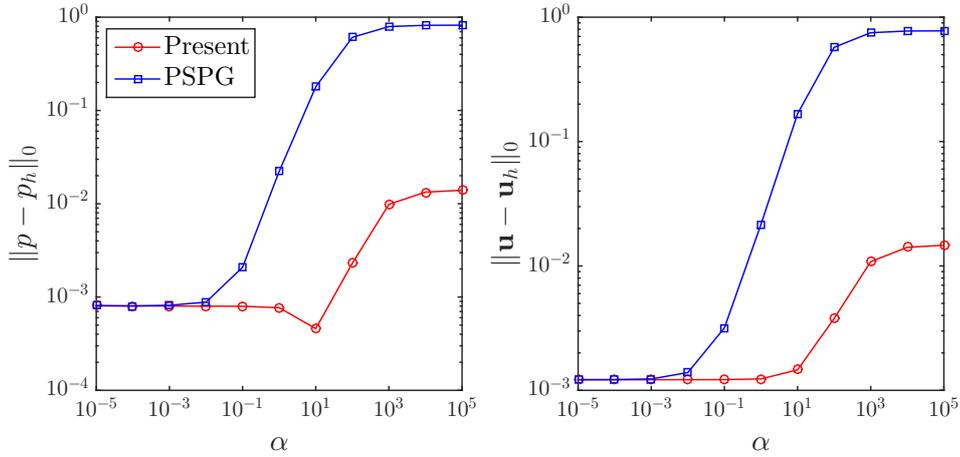
**Figure 10:** Poiseuille flow: error with respect to stabilisation parameter.
