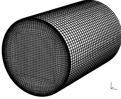
**Figure 9:** Poiseuille flow: graded mesh used for the first test case.
