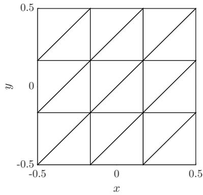
**Figure 4:** Kovasznay benchmark: coarsest mesh used in the refinement study.
