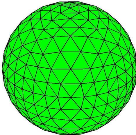
Figure 1: Third refinement level of the sphere with 512 triangles
