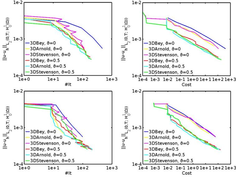
Figure 4: Comparison of AMG\_Graph preconditioned GMRES iterations (#It) (left) and costs in seconds (right) with both the uniform ( $\vartheta = 0$ ) and adaptive ( $\vartheta = 0.5$ ) refinements for  $\alpha = 1$  (up) and 100 (down).
