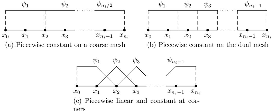
Figure 1: Possible choices for the discretization of the control
