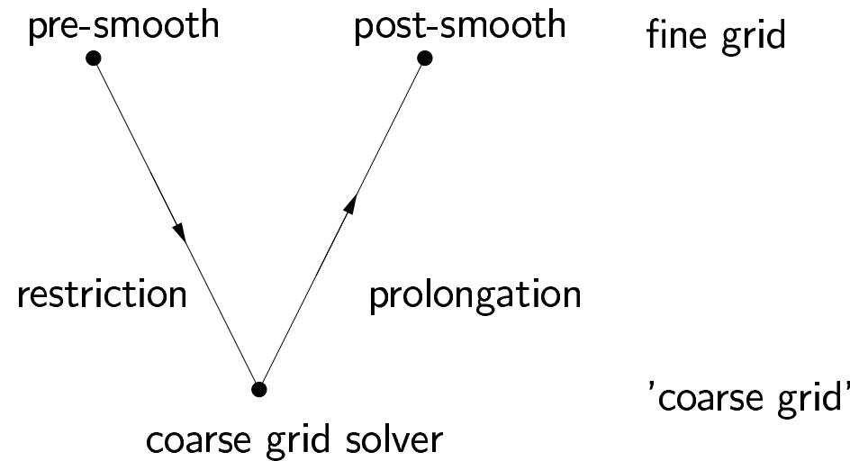
**Objective:** Construction of a multigrid cycle by using the system matrix and the right-hand side
