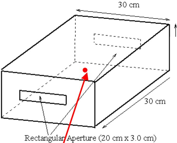
Shielding efficiency measured in the centre of the enclosure (15, 6, 15) cm.
